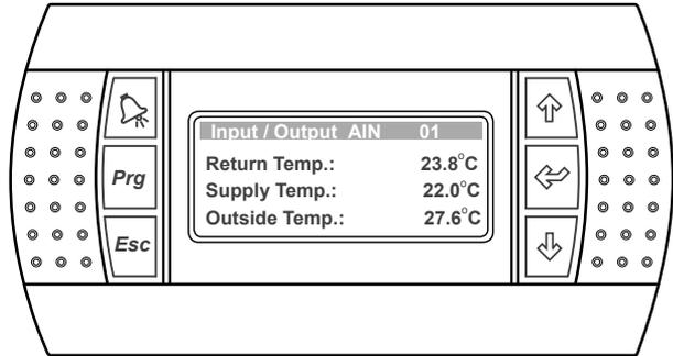
4. Press "↓" Button to scroll down into the second screen and view the operating parameters.
