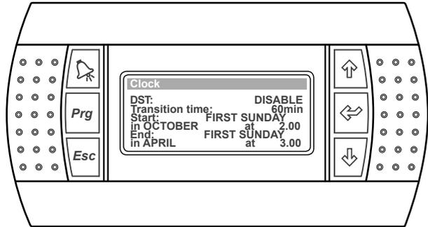
4. Press “↓” or “↵” Button to select the "**DISABLE**" Daylight Saving Time function.
