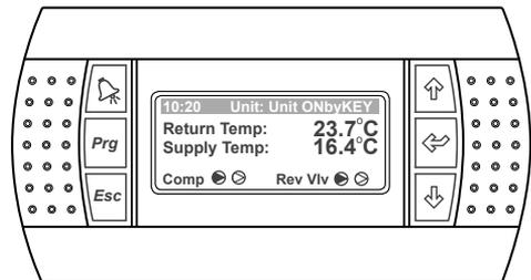
Compressor 1 & Reversing Valve 1 are On. (System in Heat Mode), first triangles are darkened
