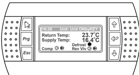
System Screen (default) provides an overview of system status, showing the Return Temperature, Supply Temperature, Compressors, Reversing Valves ON/OFF status and System Defrost indicator.
