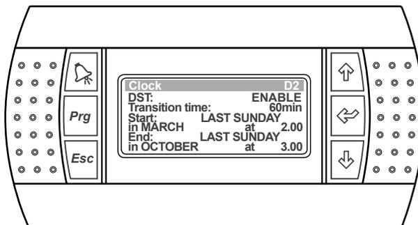
13. Repeat steps 7- 11 to set up the end of Daylight Saving Time parameters.
