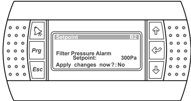
2. Press "↶" Button to move the cursor "█" down into Filter Pressure Alarm Setpoint.
