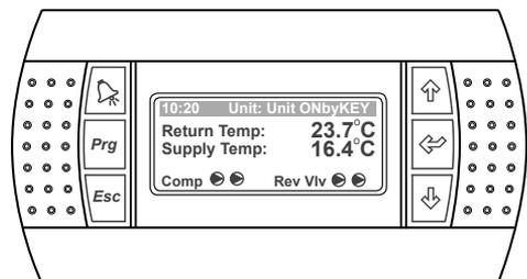
Compressors 1 & 2 and Reversing Valves 1 & 2 are On. (Systems are in Heat Mode), all triangles are darkened
