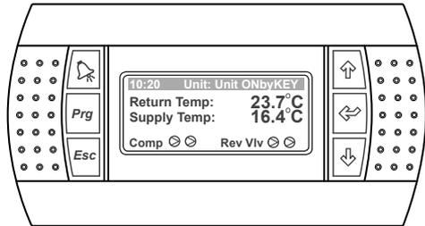
Both Compressors & Reversing Valves are Off, as indicated by clear triangles
